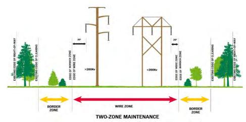
The diagram illustrates a typical right of way condition. This work is occurring within the existing edge of clearing. Your neighborhood may have a different configuration of transmission structures.
